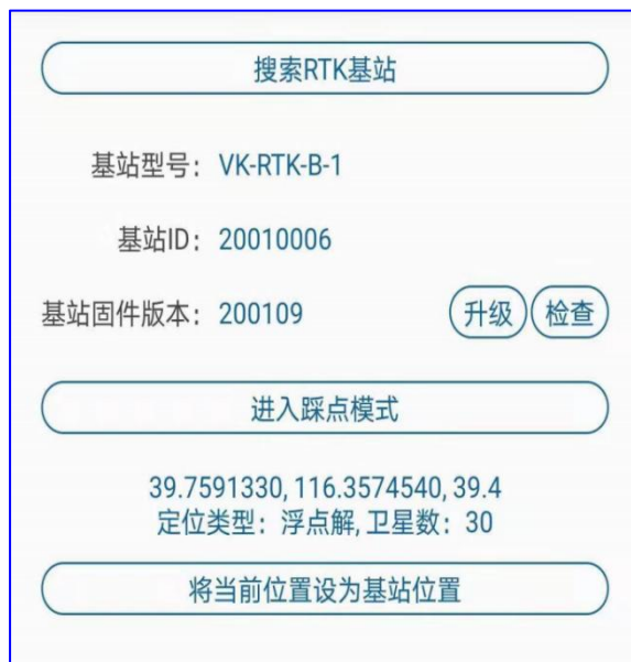
Figure: RTK base station information diagram
